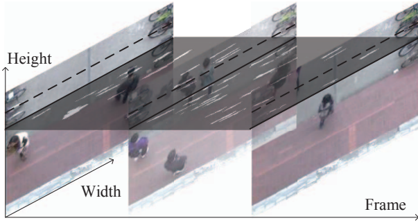
Fig. 2. The main line (solid), the associate line (dash), and the spatial-temporal matrix.
