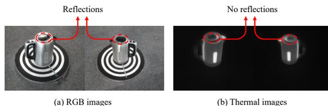
**Figure 3** Illustration of the differences between RGB and thermal images. (a) RGB images exhibit non-Lambertian effects, i.e., view-dependent light reflections, while (b) thermal images are unaffected by such effects.
